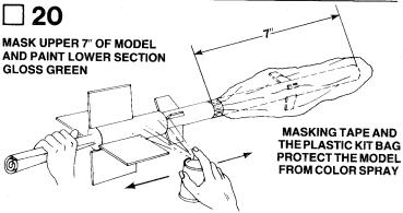
Wrap a piece of masking tape around the body 7" from the front of the tube. Be sure to remove the upper section of the model. Take the plastic bag your model came in and tape it to the masking tape on the body tube. Holding the model by the rolled up newspaper, paint the lower portion of the model gloss green. Apply paint as in Step 19 to obtain a glossy finish. Remove the masking tape and plastic bag and allow the model to dry thoroughly.
