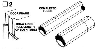
Draw straight lines to connect each set of marks made in step one on both tubes. Extend all lines the full length of both tubes. A door frame inside edge can be used as a guide as shown.
