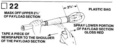
Wrap a piece of masking tape around the shoulder to completely cover it. Place a piece of masking tape along one edge of a piece of newspaper and wrap it around the balsa adapter shoulder on which
