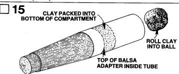
Roll the clay weight (part N) into a ball that will fit into the upper tube. Place the clay in the tube, and pack it down against the top of the balsa adapter inside the tube with a pencil or dowel.
