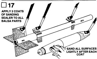
Proper application of sanding sealer makes the rocket look better and reduces drag so that the rocket will fly higher. However, this step is not essential to make a safe, attractive rocket. Apply a coat of sanding sealer to all balsa parts. When sealer is dry, lightly sand all the sealed surfaces. Repeat sealing and sanding process until balsa grain no longer shows.
