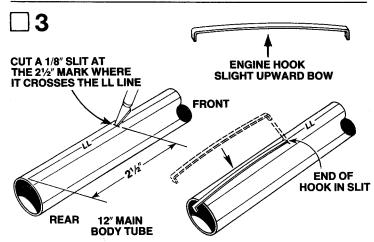
Cut a 1/8" slit in the main body tube where the 2½" mark and the launch lug (LL) line cross. Slightly bow the engine hook (part E) upward and install it in the slit.
