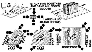
Fine-sand both sides of the balsa die-cut sheet (part G). Free the fin edges with a sharp knife, then carefully remove the die-cut fins from the sheet. Stack matching sets of fins together as shown and sand all four edges as illustrated. Lightly sand both sides of each fin. Sand the leading edges and trailing edges of each set of fins to make them round. Leave the root (body) edges sanded "flat". The root edges may be identified by careful comparison with the drawings.
