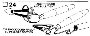
Pass the shroud line loops through the screw eye on the payload section. Pass the parachute through the loop ends and pull the lines tight against the screw eye. Tie the free end of the shock cord firmly to the screw eye. A square knot or strong double knot should be used.
