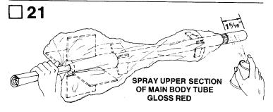
Wrap a piece of masking tape around the main body tube 15/16" from the front of the tube. Tape the kit bag over the portion of the model behind (to the rear) of this tape line. Spray the upper 15/16" of the main body tube gloss red. Remove the tape and bag and allow to dry completely.
