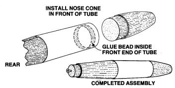
Run a bead of glue around the inside of the front of the tube and push the nose cone (part O) into place tight against the top of the tube. Allow the completed assembly to dry (thoroughly).
