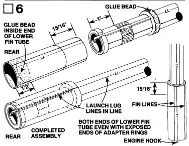
Test fit the lower fin tube on the rear end of the main body assembly. Align the launch lug line or the fin tube with the launch lug line on the main body tube. This should also align the launch lug line with the en-
