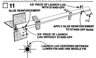
Cut two 3/8" pieces from the launch lug (part I). Glue <u>one</u> of the launch lugs to one of the standoffs found on the balsa sheet. <u>You will not need the other standoff!</u> Glue the launch lug with the standoff 1 1/2" from the front of the main body tube. Glue the other launch lug directly to the fin
