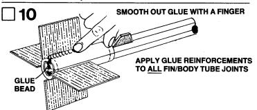
Apply a bead of glue to both sides of one fin/body tube joint and smooth out with your finger, being sure to wipe off excess glue. Repeat with all twelve fins. When all glue reinforcements are done, rest the model on a table edge as you did in Step #9.
