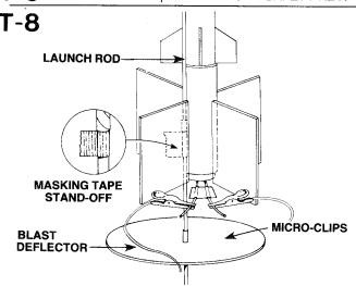
Slide the launch rod through rocket launch lugs and place rocket on launch pad. Make sure the rocket slides freely on the launch rod. Clean the micro-clips and attach them to the igniter wires. Arrange the clips so they do not touch each other or the metal blast deflector. Attach clips as close to protective tape on igniter as possible.
